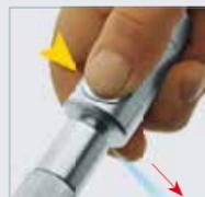
**1 Impulsion 1:** automatic decompression of the downstream hose, with the plug continuing to be held in the part position in the coupling.
